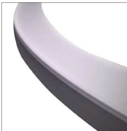
Kinetically sprayed zinc on a large-size SKF ring
