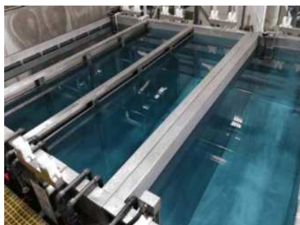
Water rinsing tanks in an SKF coating facility
